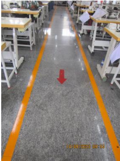
Exit pathway marking.JPG
